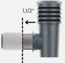
STEP 4 : Insert the vent into the opening maximum so that the turbine or vent rings are 1,1/2" away from the wall. Secure it in a vertical and horizontal position with shims. Bubble levels are built in for correct and easy setting.
