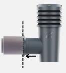
STEP 5 : Foam the place between the intake pipe vent and the opening in the wall with fast cure foam sealant.
