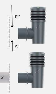
STEP 1 : Before making the opening and installation, choose the place of installation and making the opening so that there is 12" space above the opening and 5" below the opening.
